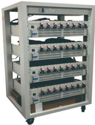
5V60A charging and discharging cabinet
